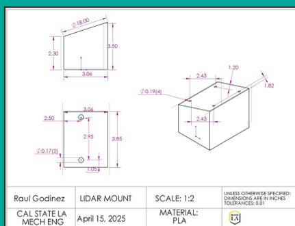
SolidWorks Drawing: LiDAR Mount
