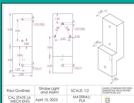
SolidWorks Drawing: Strobe Light & Alarm Mount
