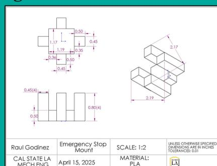
SolidWorks Drawing: Emergency Stop Button Mount
