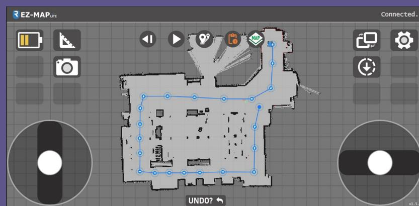
A complete map of the Electronics Lab using the LiDAR to scan and map the area. Uses the sonar to avoid any obstacles by using the implemented collision detection. Uses pinpoints to navigate throughout the area
